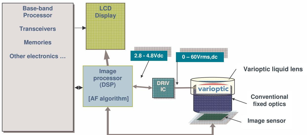
To drive the liquid lens, either the DrivIC 60 or VPS-048m mini-board can be used. The DrivIC 60 is aimed for high volume designs.
